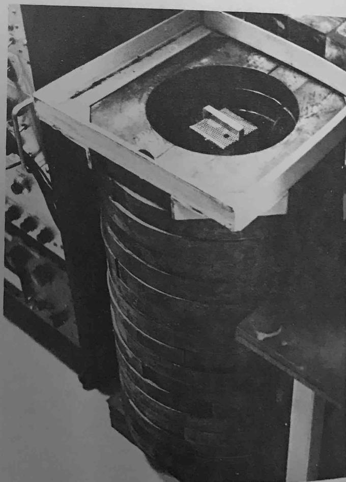
Mr. Stephen Walsh of the Radioecology Division shows(left) samples of lead ingots extracted from a Peruvian mine, dated 1535, which were found off the west coast of Puerto Rico. Some of the lead was melted down for use as a cylindrical radiation shield in the Marine Biology program(right).
