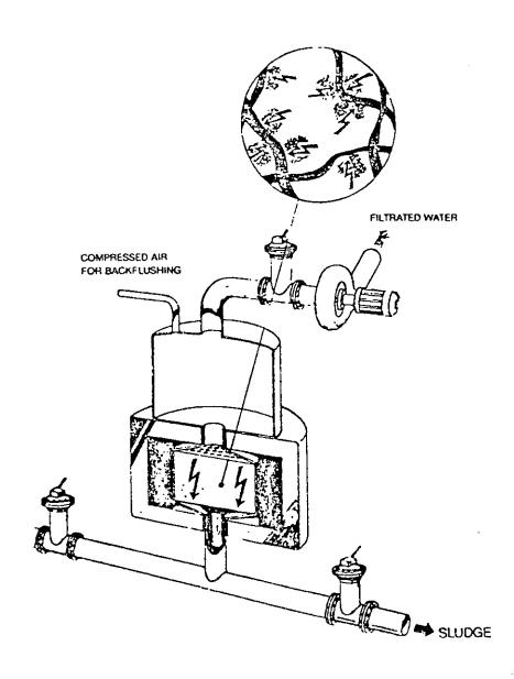
High Gradient Magnetic Separation and Filtration Applications
